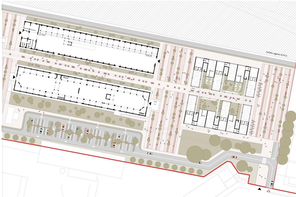
Figure 15: Floor plan of the project. The solution adopted seeks a possible balance with the pre-existing buildings by interpreting their position, proportions and densities
